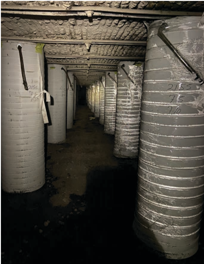
J-CRIB®, a pumpable standing support, provides significant strength and logistical advantages over traditional coal mine standing support.
